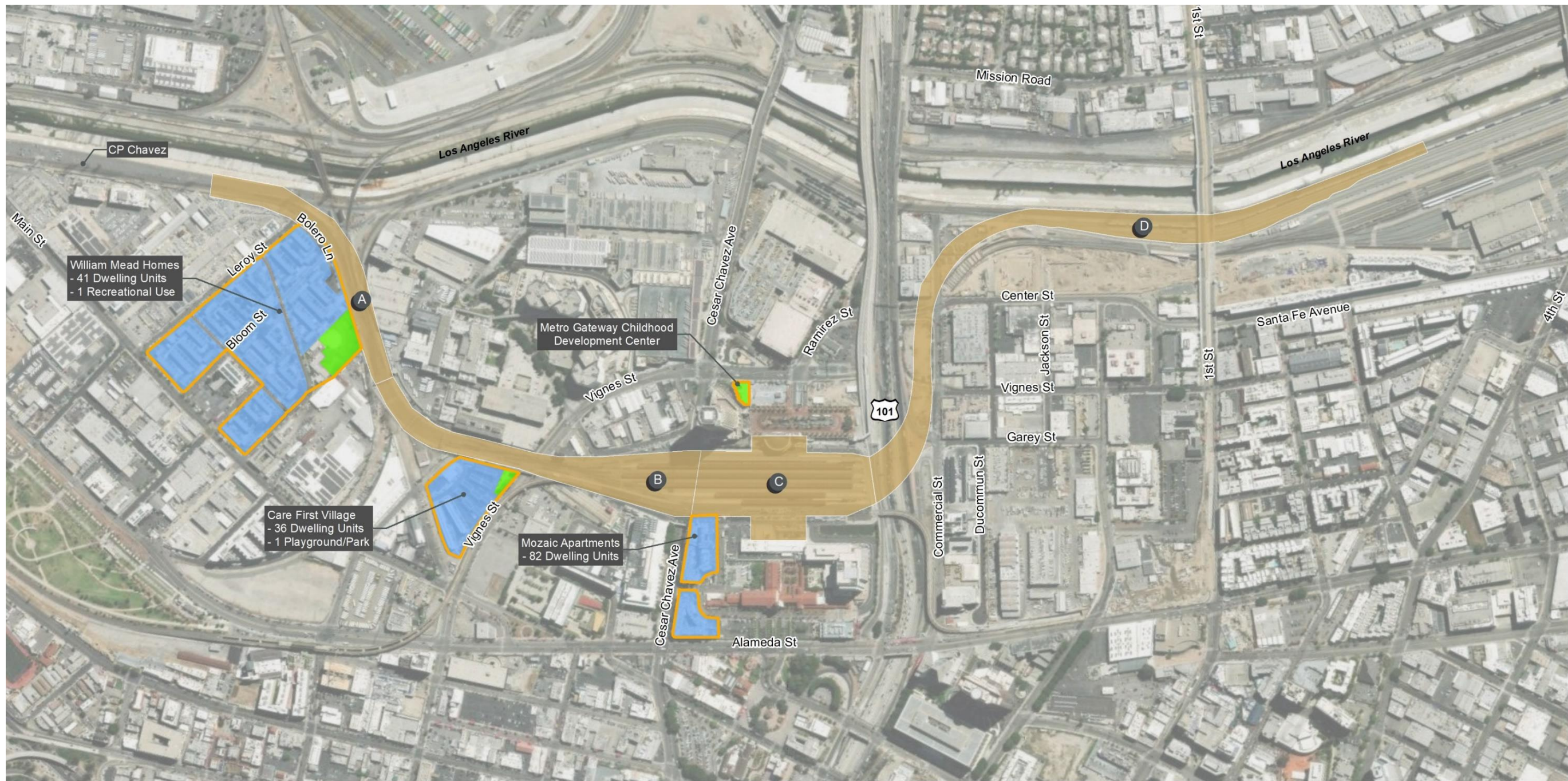
Figure 3.6-12. Land Uses Subject to Construction Noise Exceeding City 75 dBA Limit
