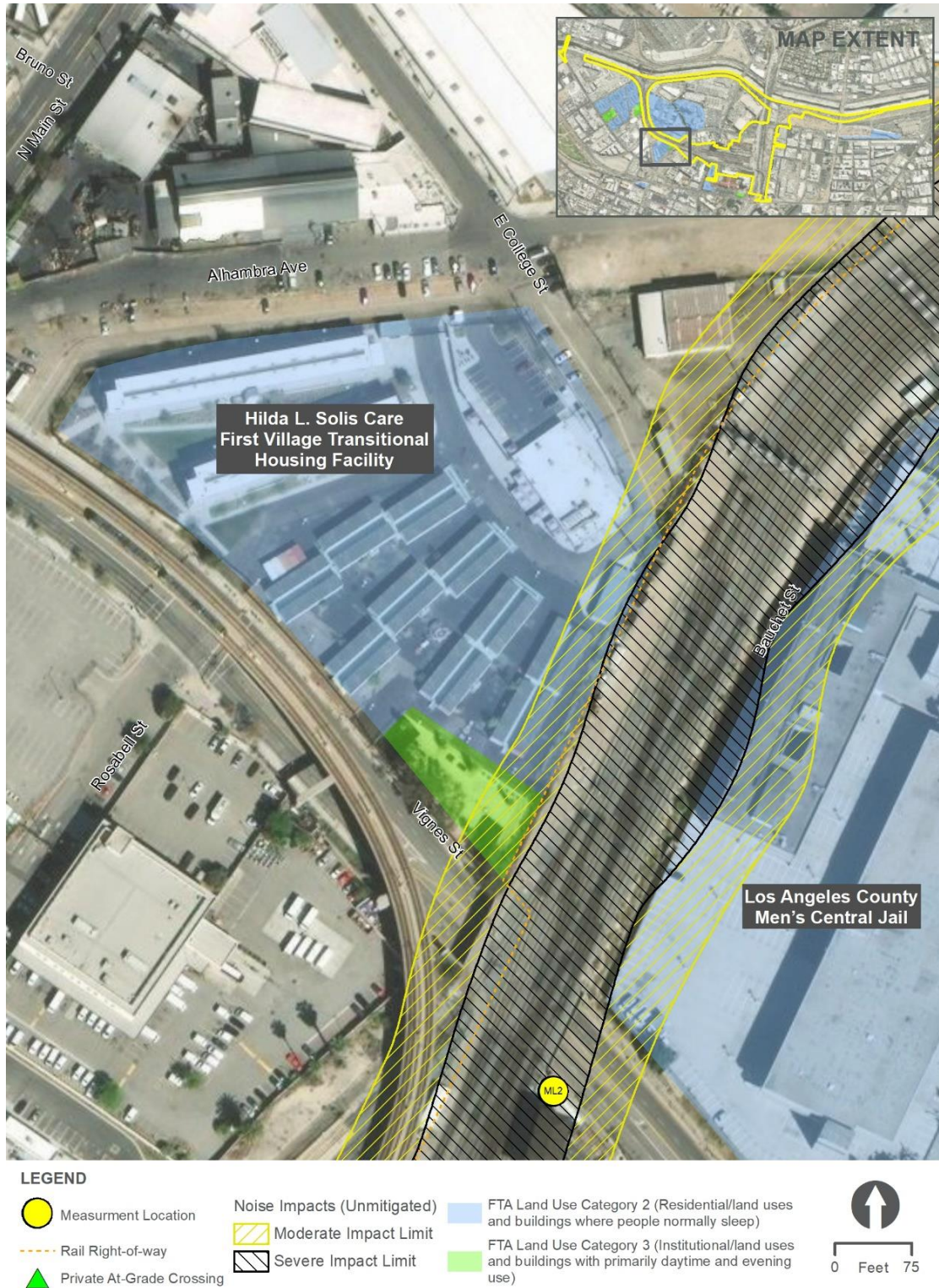
Figure 3.6-16. Noise Impact Areas at the Care First Village – Build Alternative without Mitigation (2031 Condition)
