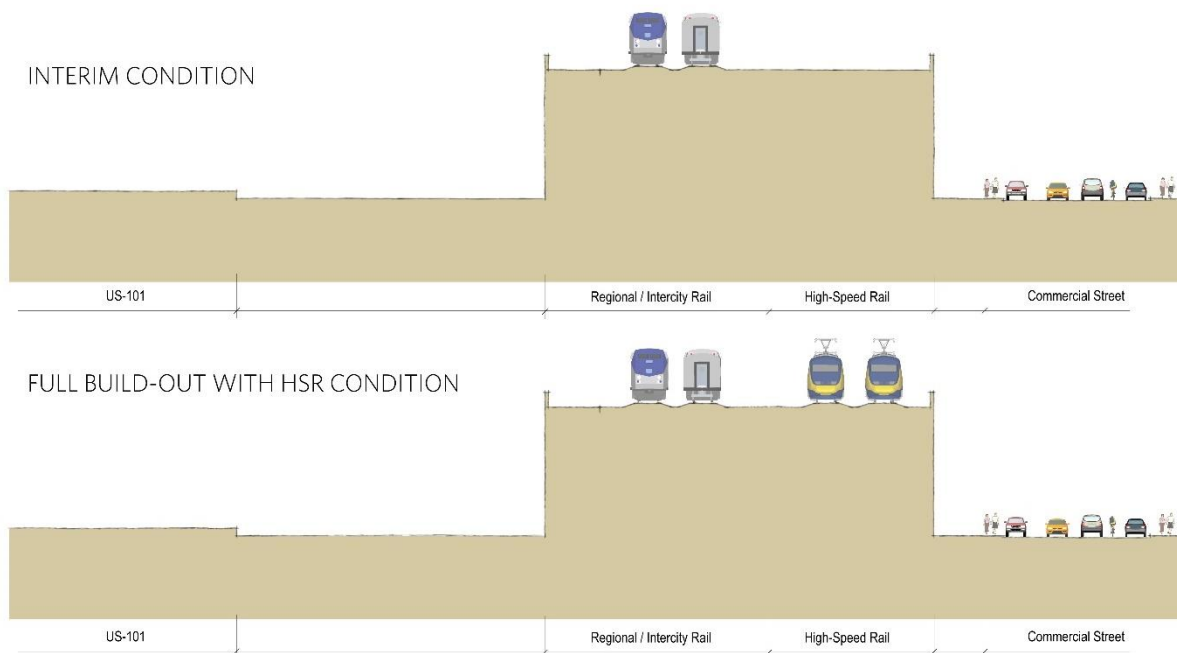
Figure 2-19. Common Run-Through Track Embankment South of US-101 (Looking East)
