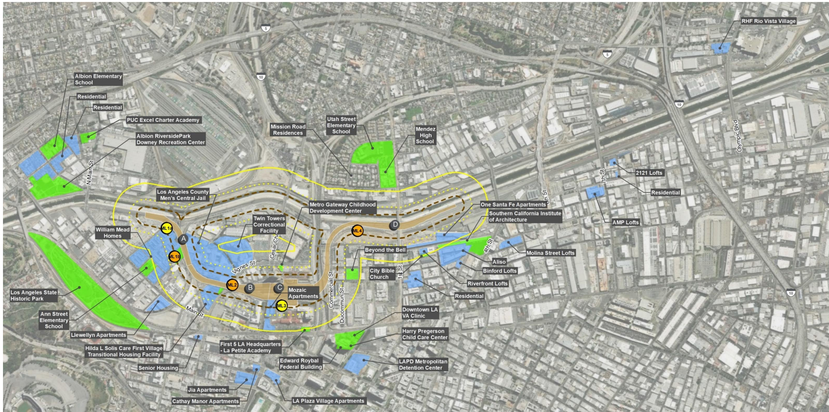
Figure 3.6-4. Noise- and Vibration-Sensitive Land Uses, Community Noise and Vibration Measurement Locations, and Sensitive Receptor Clusters
